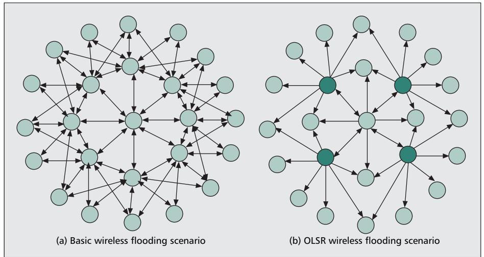
■ **Figure 6.** a) Basic wireless flooding scenario and b) OLSR wireless flooding scenario.
