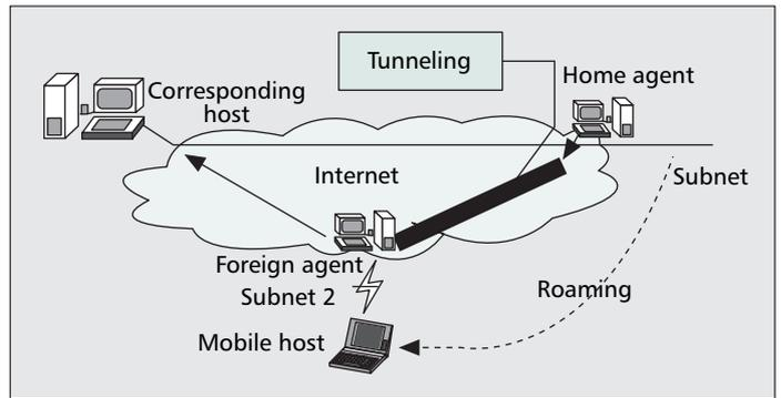
■ Figure 1. Mobile IPv4 architecture.
