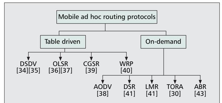
Figure 5. Mobile ad hoc routing protocols classification.
