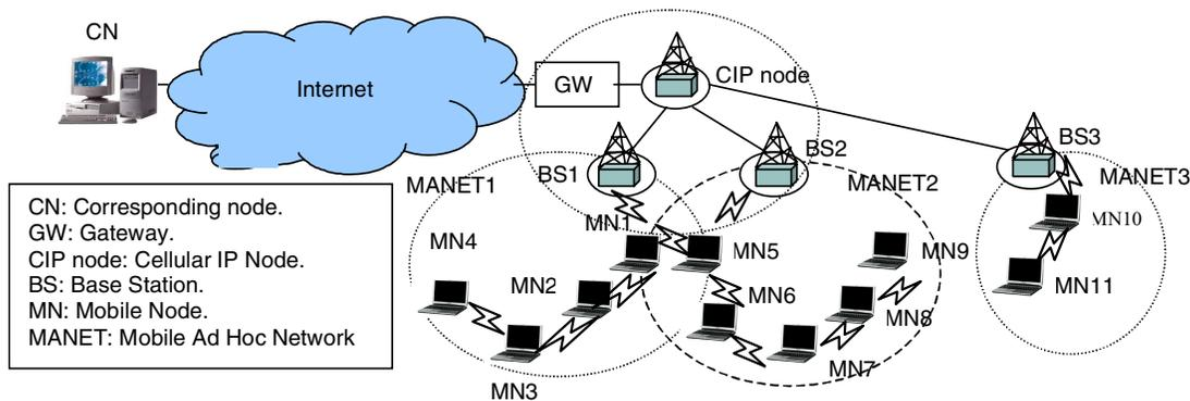
**Figure1: Integrated network architecture.**
